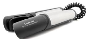
The Vernier Go Wireless Heart Rate consists of a pair of wireless hand grips that measure heart rate on a mobile device. It is ideal for continuously monitoring heart rate before, during, and after exercise or while a person is stationary. Data are wirelessly transmitted to iPad<sup>®</sup>, LabQuest<sup>®</sup> 2, or other mobile devices that are Bluetooth<sup>®</sup> Smart Ready.
