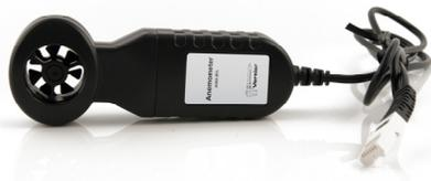
The Anemometer is a device for measuring wind speed.
