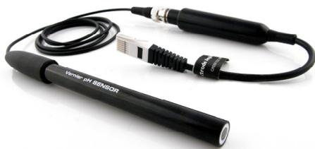
The Tris-Compatible Flat pH Sensor measures the pH of a solution or semisolid. Because the glass membrane is flat instead of a bulb, it is more durable, easier to clean, and allows for flat surface measurements and smaller sample sizes. It features a sealed, gel-filled, double-junction electrode, making it compatible with Tris buffers and solutions containing proteins or sulfides. The attached Electrode Amplifier stores a custom calibration.
