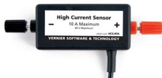
The High Current Sensor is used to measure current in the range of  $-10$  to  $+10$  A. The sensor uses a Hall Effect chip, so that it does not add a resistive element to your circuit. A metal shield over the Hall Effect chip reduces the influence of external magnets. A replaceable fuse protects the equipment and circuit. Use the sensor in experiments that involve currents larger than 1 A, such as solar panels, hand generators, etc.
