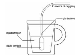
Place a Styrofoam cup into a coffee mug and fill it 3/4 full of liquid nitrogen. With the oxygen gas flowing, submerge the bulb of the pipet in the liquid nitrogen. In less than 10 minutes, the bulb of the Beral pipet should be more than half full of blue-colored liquid oxygen!
